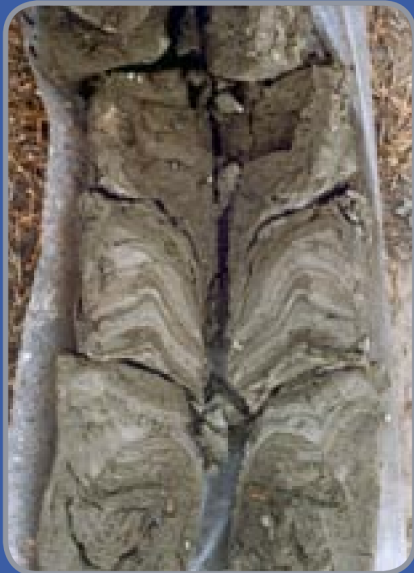
■ Mine tailing core sample
